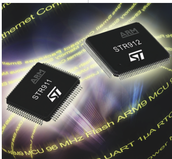
The STR910F series of ARM9E-based microcontrollers combine Ethernet, CAN 2.0B, and USB-FS support; as much as 96 kbytes of SRAM; and as much as 544 kbytes of flash.
